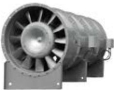
ZAXN Axial Fans for car park ventilation and higher pressures (2 AXN in line impeller with 6/9/12 blades)
